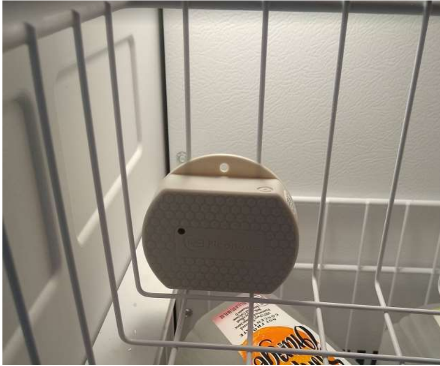
Figure: SN400 Magnet Mount Inside Refrigeration Equipment (affix to steel shelving)
