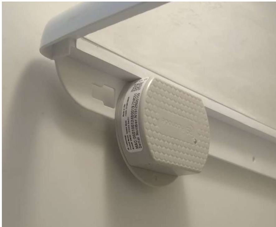
Figure: SN400 Magnet Mount Inside Refrigeration Equipment (probe ports protected from spills by shelf)
